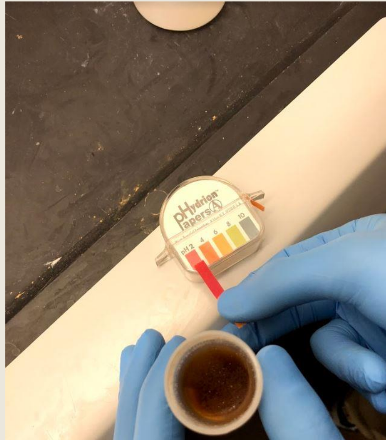
Figure 8. Acidic pH of treated corn after centrifuging
