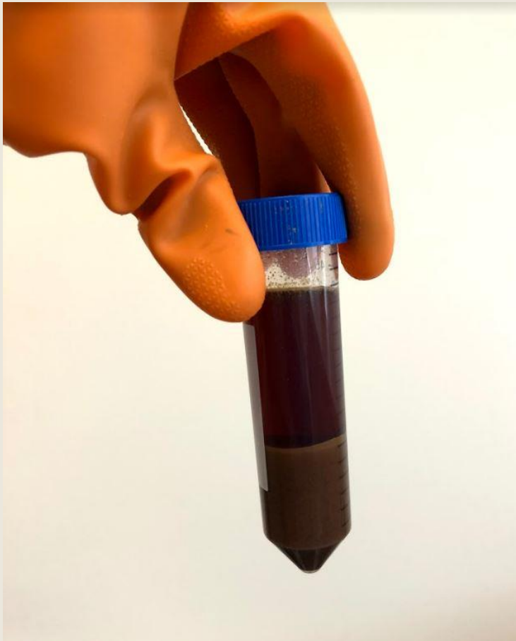
Figure 7. Corn treated with nitric acid and centrifuged
