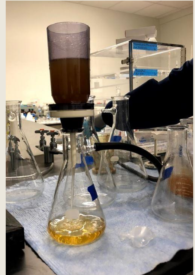
Figure 13. Solid corn filtered out of solution
