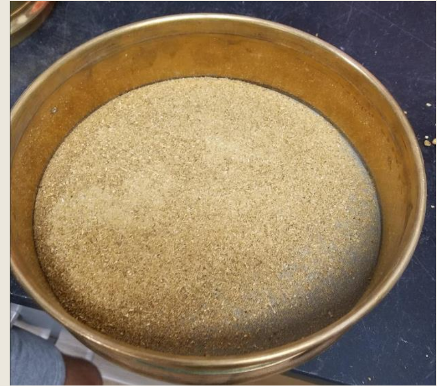
Figure 6. Pulverized corn passed through No. 60 sieve (250 microns)
