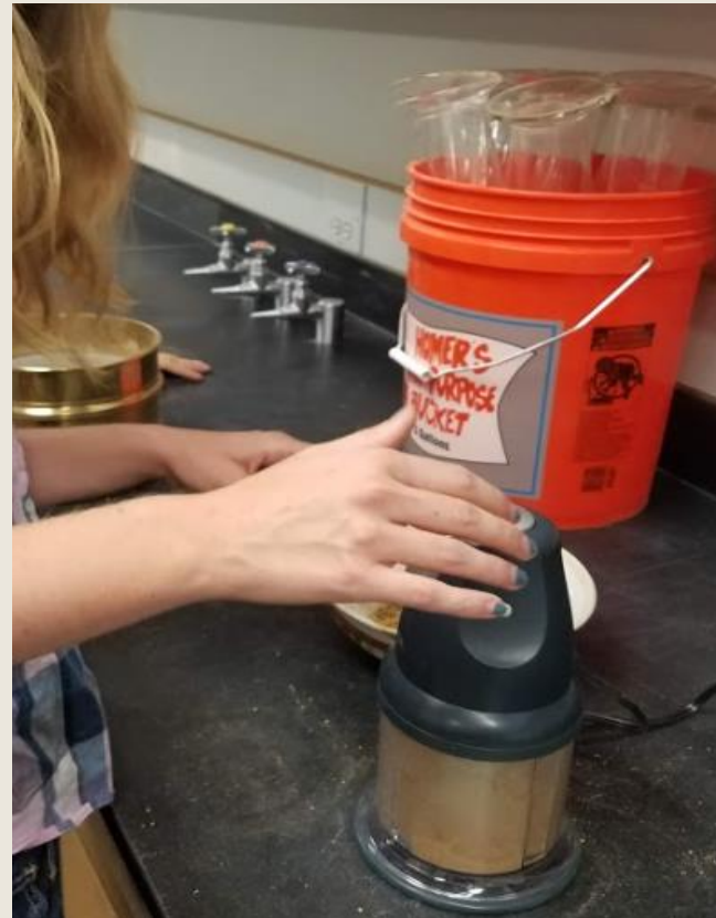
Figure 5. Dried corn cobs pulverized in a food processor
