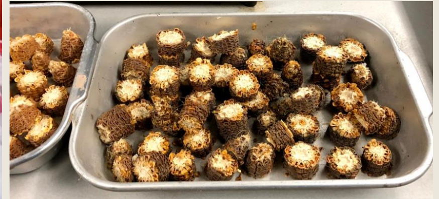
Figure 3. Dried corn cobs after being placed in drying oven for 24 hours at 100 °C
