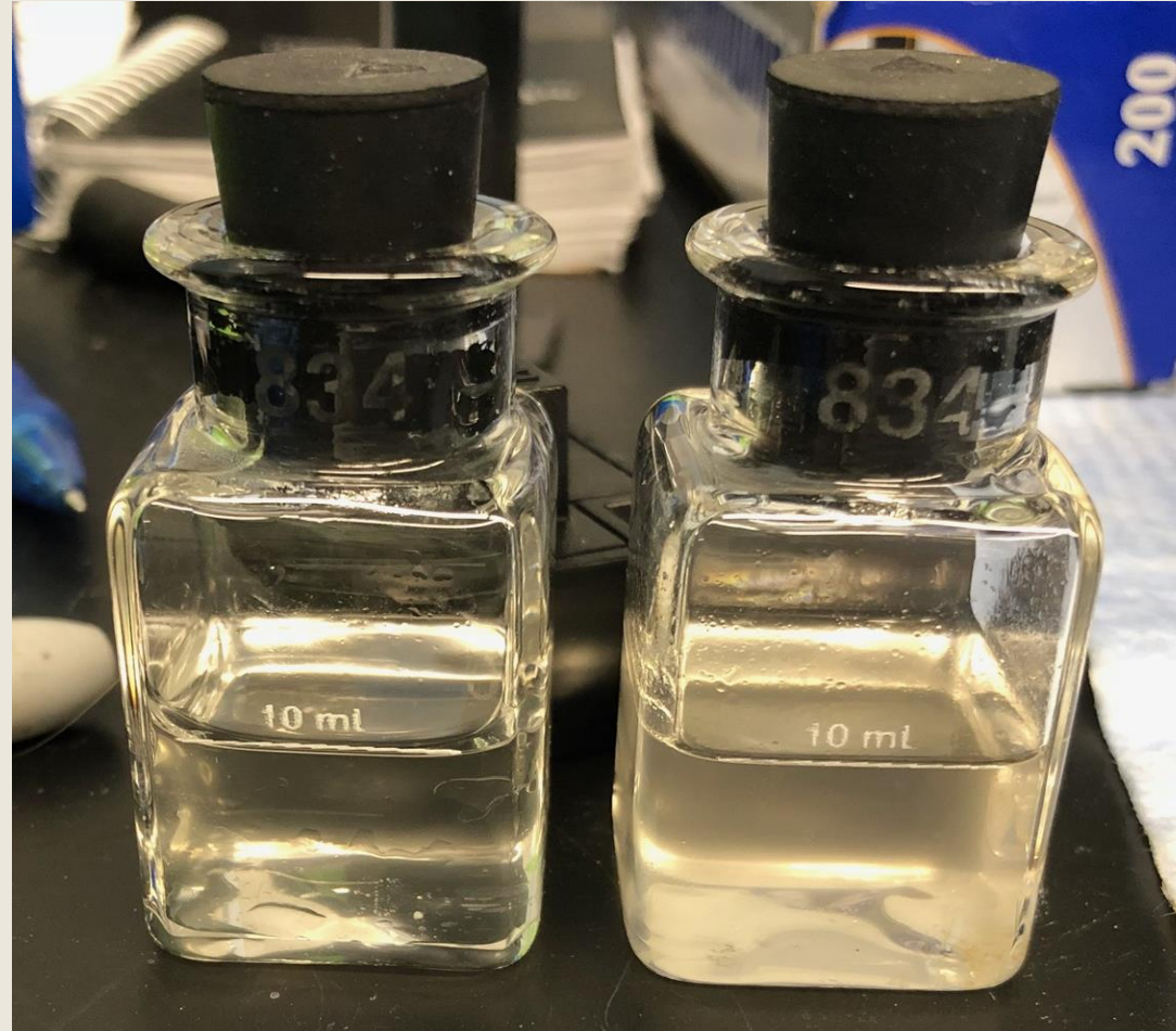
Figure 21. Cloudiness of samples interferes with cadmium readings
